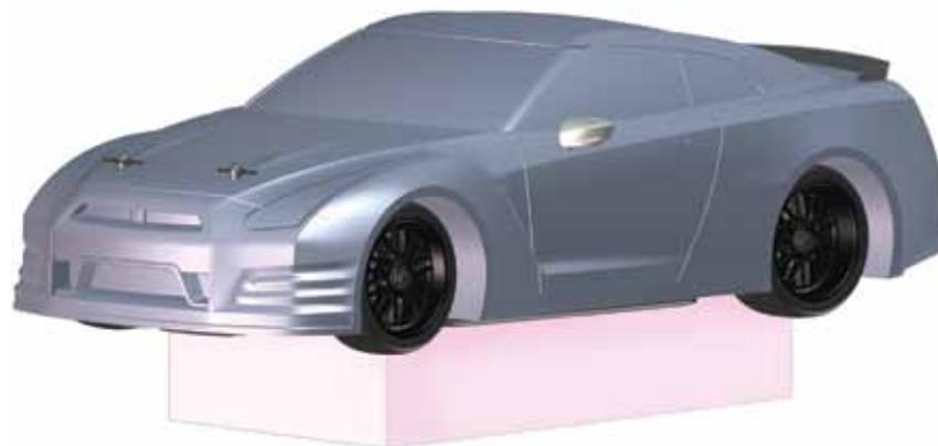
Perform a control test with the vehicle wheels off the ground. If the wheels rotate after the vehicle is powered ON, adjust the “TH. Trim” knob until they stop. To make the wheels move forward, pull the trigger. To reverse them, wait for the wheels to stop, then push the trigger. When moving forward, the wheels should maintain a straight line without any steering wheel input. If not, adjust the “ST. Trim” knob so the wheels maintain a straight line without having to turn the steering wheel.
